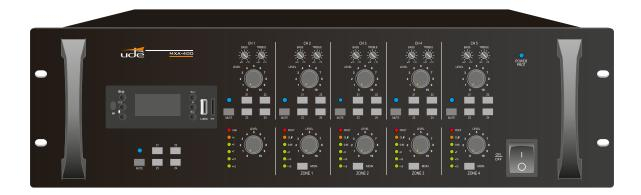
The MXA-400 allows audio switching from 5 inputs to 4 amplified/line audio outputs, amplified output with a range of in  $4\Omega$  / L70V and L100V with 120W. rms each one. High performance, and an easy way due to the frontal switch buttons. All audio inputs have volume and bass / treble control.
