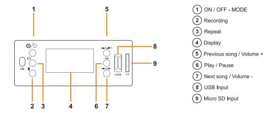
1. Power on the MP3 module by pressing the ON / OFF button next to the display for 2 seconds.
