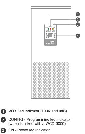
A RJ-45 socket for WCD-3000 linking.
